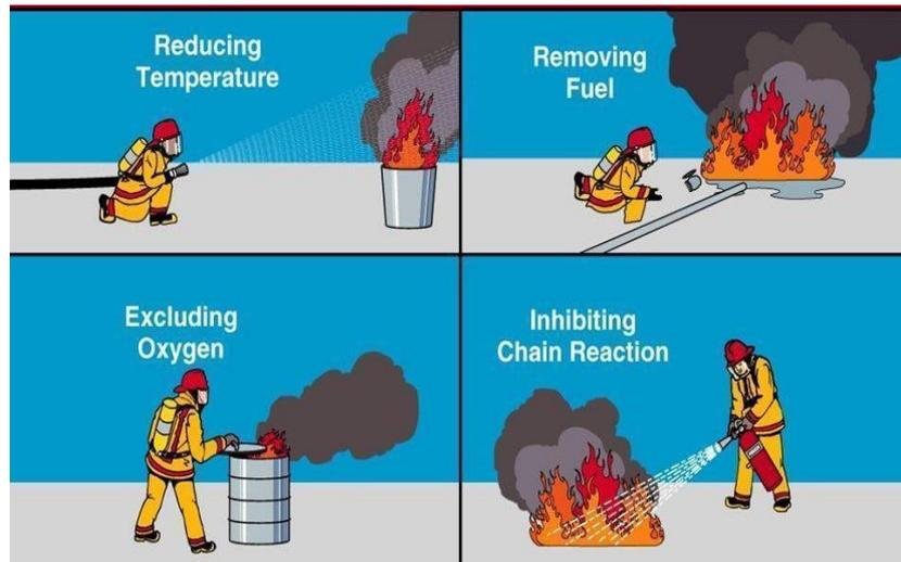
Figure 4.3. Fire extinguishing techniques.
