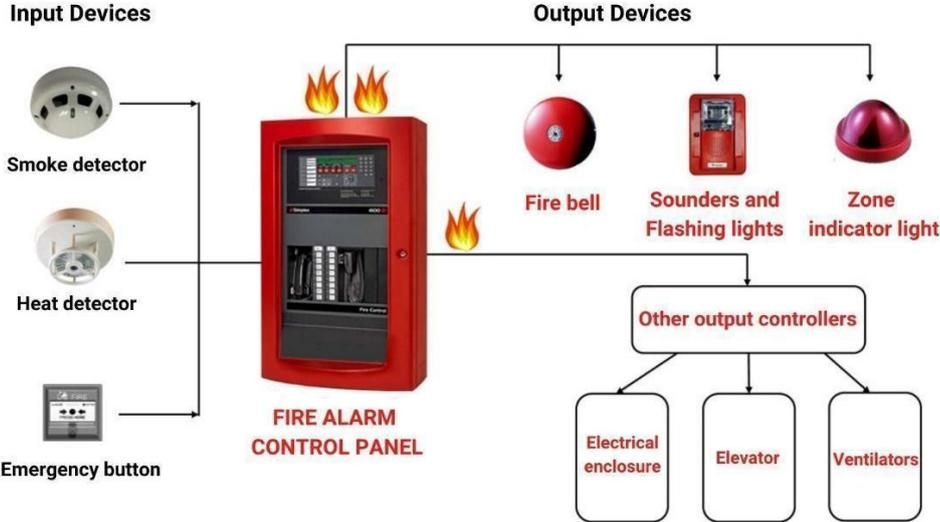
Figure 4.7. Fire alarm control panel.
