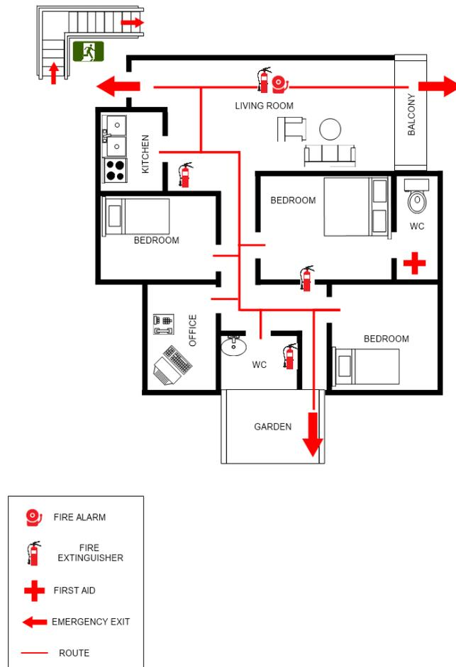
Figure 4.9. Evacuation plan (sample).
